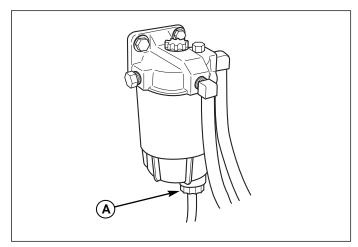
Figure 12. Drain Fuel Filter
